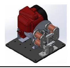
In this course the flexible "DeskTop Dynamometer" is used to explore many aspects of Engine Testing. The DeskTop Dynamometer comes with a Honda GX35 Gasoline Engine, and dynamometer controller, together with software for displaying and logging data from the engine. Various experiments are described, along with theoretical considerations, and then demonstrated live, including analysis of the resulting data.
