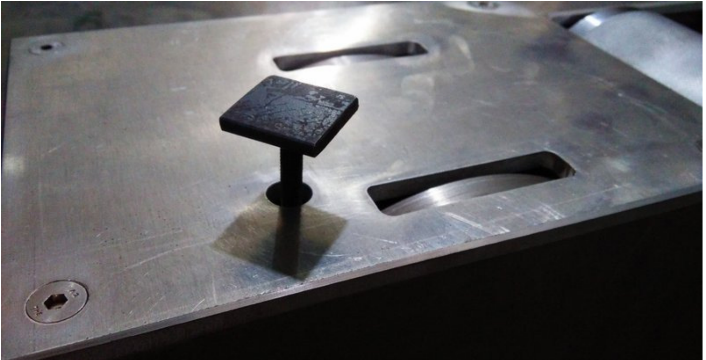
This view shows the Calibration Weight Platform screwed into the internal Load Cell for calibration.
