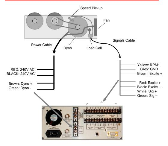
The Controller should be is powered from a clean AC line power source.
