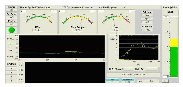
In general the display is self explanatory. The various meters can be re-scaled by changing the range limit numbers in the upper corners of the meters. The graphs can be cleared or rescaled by right clicking on the graph, and following prompts. Analog input channels voltage values are displayed and graphed in the lower logging graph.
