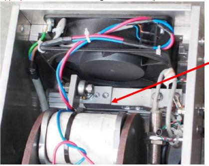
Screw Calibration Weight in to this hole
