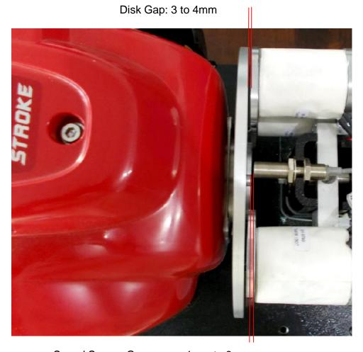
Speed Sensor Gap: 1mm to 3mm
