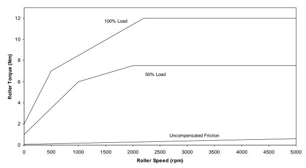
Torque is limited by the available voltage from the dyno at low speeds. At higher speeds, the torque is relatively constant as the dynamometer operates in a current (torque) limited mode. The roller speed should be limited to 5000rpm to avoid damage to the dynamometer. The lower limit of torque is the total friction. The safe area of operation is anywhere between the frictional curve and the 100% load line. For reference a 50% load line has been given.
